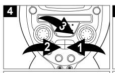
Press the Skip/Search (►►I) ① or (►►I) button ② to select the first track that you wish to program. When the desired track number appears in the display, press the PROGRAM button ③ again.
